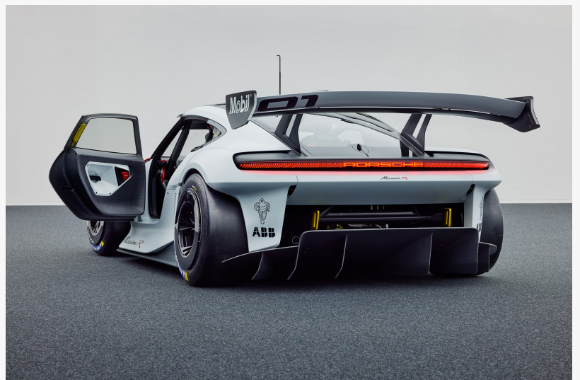
Many of the add-on parts on Porsche's visionary fully electric Mission R concept car are made using Bcomp's natural fibre reinforced plastic (NFRP). The natural fibre material can be seen on the car's exterior, such as the front splitter, the doors, the s
