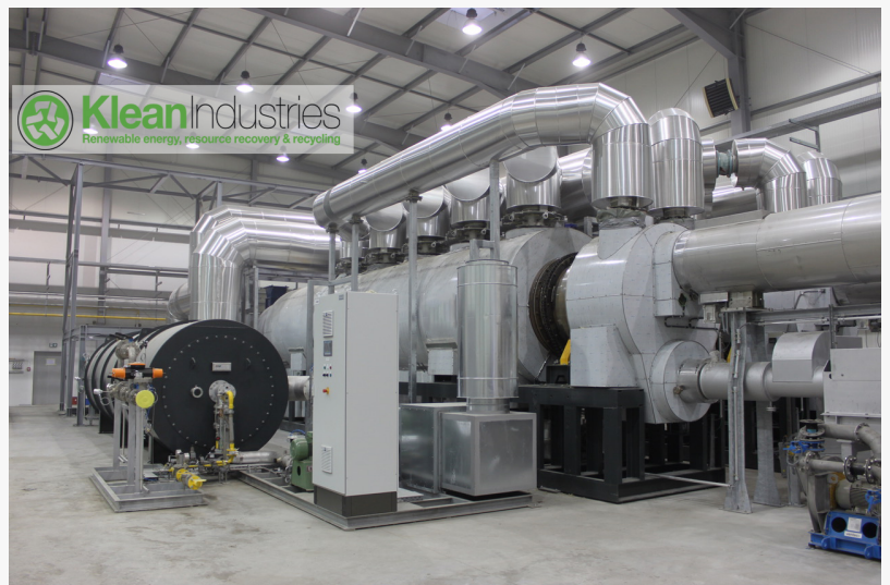
Klean Industries Modular Technology for End-of-Life Tyre Pyrolysis Recycling System
