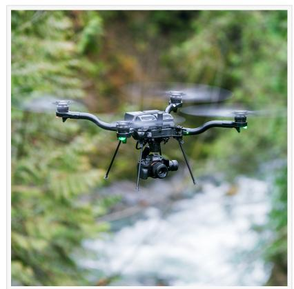
Freefly's new NDAA-compliant Astro UAS leverages a Doodle Labs mini Mesh Rider Radio as its on-board datalink.
