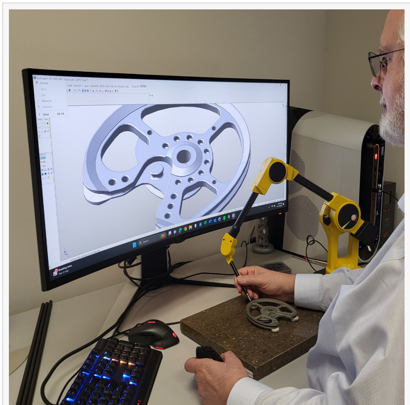
A desktop reverse engineering station with KeyCreator CAD and MicroScribe CMM
