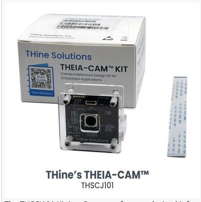
The THSCJ101 Kit is a Camera reference design kit for embedded camera applications using the NVIDIA®
