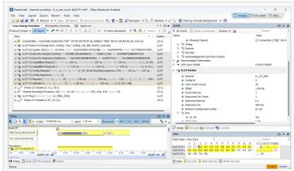
A log file of channel sounding protocol transactions created with the Bluetooth Vanguard protocol analyzer from Ellisys
