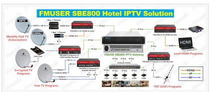
FMUSER's hotel IPTV solution offers versatile content sources, including UHF and satellite signals (paid TV programs like Canal+ and DSTV, as well as free TV programs like Arabsat, Ethiosat, Hotbird, and Nilesat), along with encrypted TV programs through
