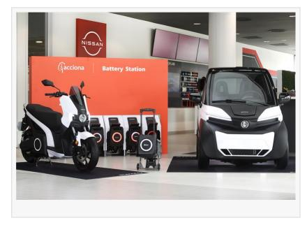
The S04 comes in two models – the L7e and the L6e. The L7e is equipped with two batteries and offers 14kW of power, reaching 85km/h with a range of 149 kilometers. The L6e, which can be driven without a driving license, operates with one battery and 6kW of power, reaching a maximum speed of 45km/h.
