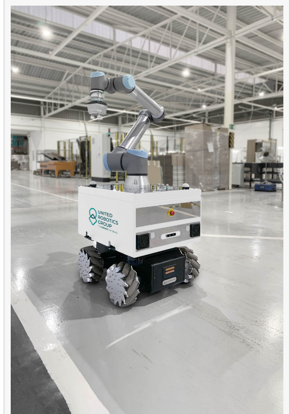
Kairos robot is a collaborative mobile manipulator
