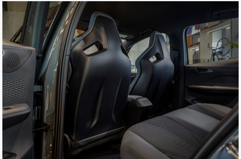
CUPRA's Born VZ electric vehicles' new bucket seats feature natural fibre composites from Bcomp
