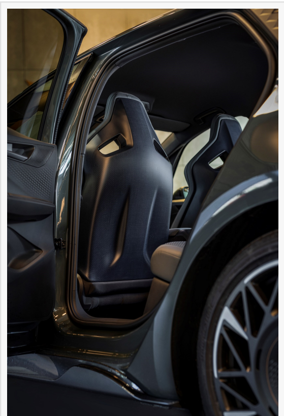
CUPRA's Born VZ electric vehicles' new bucket seats feature natural fibre composites from Bcomp
