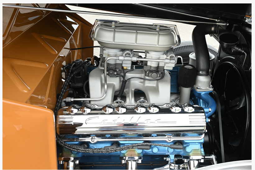
A Vintage Cadillac engine was detailed and updated with modern electronic fuel injection.
