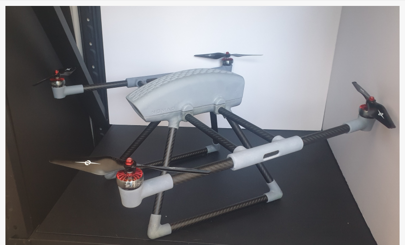
1st generation resin drone assembled for fit test before undergoing sandblasting for final ceramic coating. (Image Credit: Phillip Keane)
