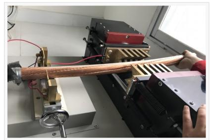
Bare copper conductors are tested to very strict specifications at the time of inspection to ensure cable quality.
