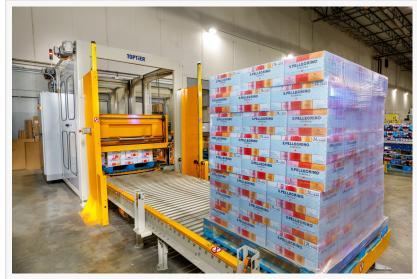
Once through the variety pack line, pallets of shrinkwrapped carton packs are sent through an automated palletizer which seals the pallet for shipment
