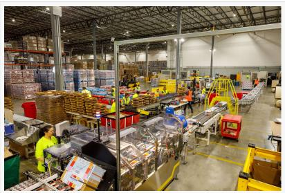
Bettaway added more speed to its beverage packing line, incorporating a new, automated carton assembly unit that takes flat cardboard pieces and folds and seals them into cartons.
