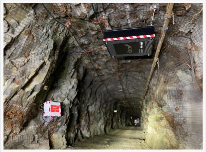
Ideon's new in-mine imaging solution installed at the NORCAT Underground Centre. With a few of these detectors, mines can map density at metre-scale precision over billions of cubic metres of rock – helping accelerate time to market for critical minerals.
