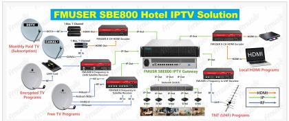
FMUSER's hotel IPTV solution is compatible with versatile content sources, including local HDMI, UHF, Satellite Signals (paid TV programs like Canal+ and DSTV, as well as free TV programs like Arabsat, Ethiosat, Hotbird, and Nilesat).
