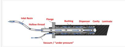
The patent covers the process of infusing epoxy resin into the bushing via an inlet tube. Using vacuum the resin is then distributed evenly around the outside of the bushing fixing it in place.
