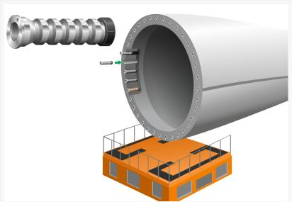
Following precision machining and extraction of the damaged bushing, the patented bushing is inserted into the rotor blade root which has been placed in a repair environment within the wind park
