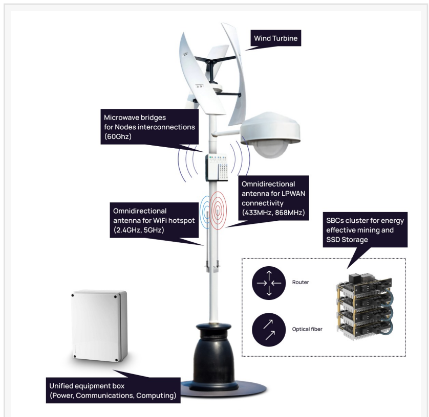
Generalized architecture of the Luna° Mesh Base Node
