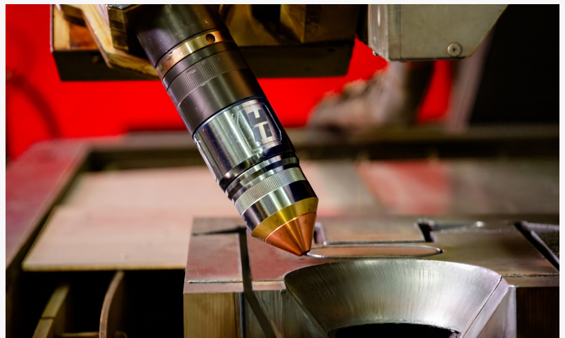
Provides a smooth surface, low angularity, and minimal to no dross for clean parts off the table
