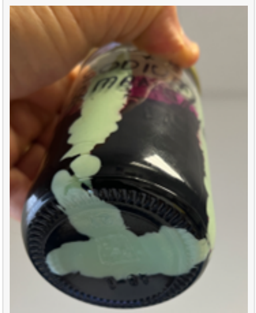
LOX-8 Thread Sealant in Sodium Permanganate after 350+ Hours
