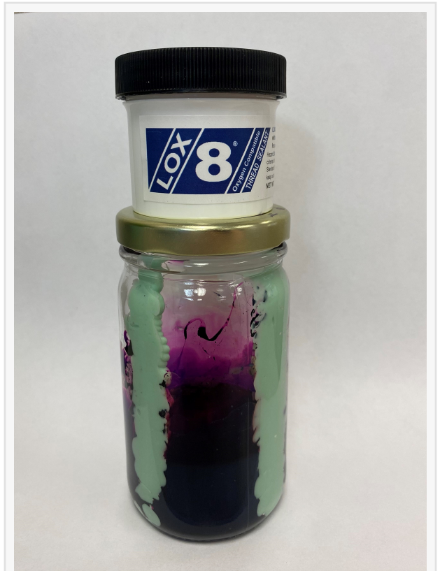
LOX-8 Thread Sealant and Sodium Permanganate
