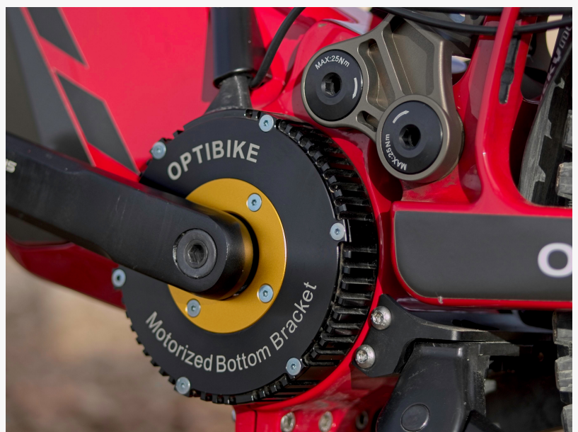
Optibike RIOT with Powerstorm HT motor
