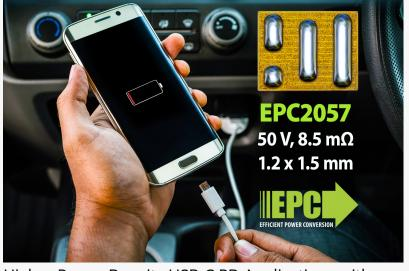
Higher Power Density USB-C PD Applications with New 50 V GaN FET in Tiny 1.8 mm2 Footprint from EPC
