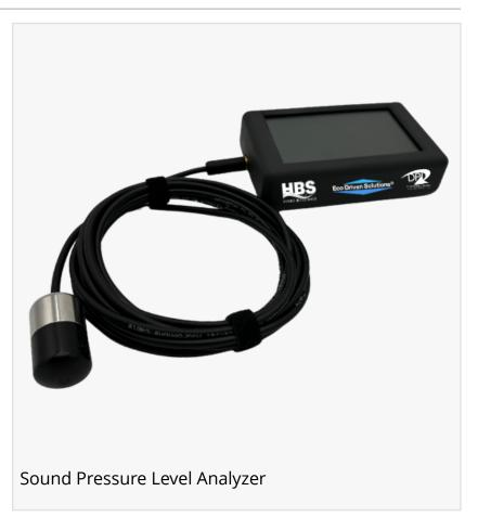
management professionals to make an immediate assessment with actionable data. The new SPL Analyzer comes standard with a USB Type-C interface for FREE firmware upgrades and audio file transfers, boasting ample built-in memory to capture and retain audio recordings in .wav format.
