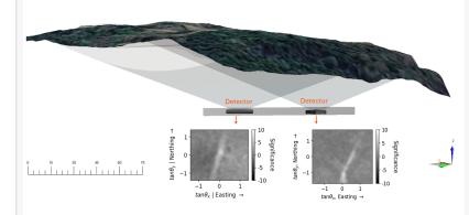
Positions of the in-mine imaging equipment in the mine adit, the fields of view covered as the muon detectors image upwards towards the surface, and the radiographs outlining a low-density anomaly corresponding to the conveyance tunnel above.
