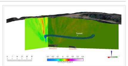
Section view of the density model showcasing the linear tunnel feature (blue), as imaged above the Ideon muon detectors positioned in the mine adit beneath, mapped to metre-scale accuracy. Note that the resolved tunnel density is 0 g/cc.
