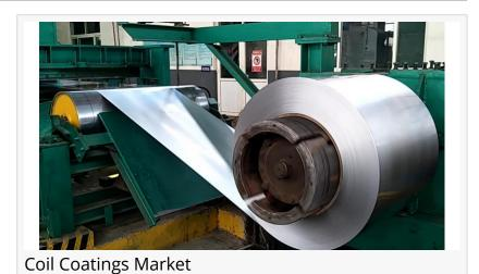
Coil coatings are surface coatings applied to metal coils, especially hotdip-galvanized steel and aluminum
