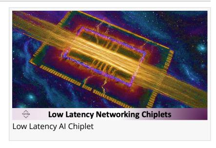
Chiplets features low latency of sub 60nS for 100G traffic with ability to do port to port switching in under 150nS. It is designed for 12nm node and targeting latency sensitive markets such as industrial, aerospace, networking and financial markets.
