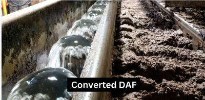
SAF® Generators produce aphrons which attach to and float particles out of water to be removed.
