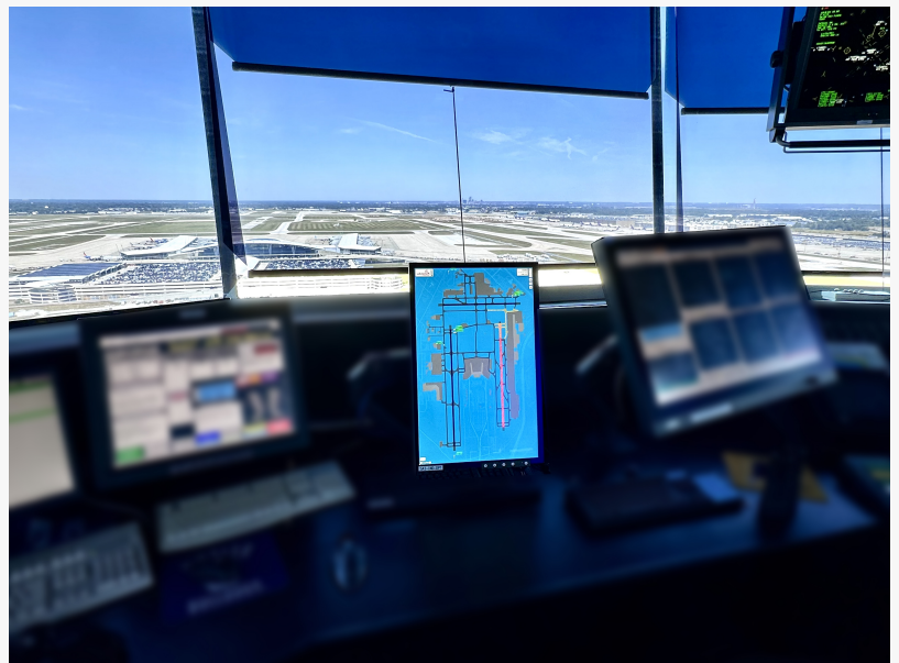
Surface Awareness System at IND
