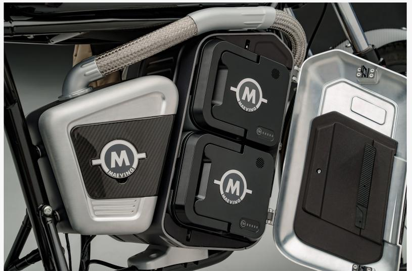
The Maeving RM1S powerpack can be charged in situ or removed to charge at a wall socket.
