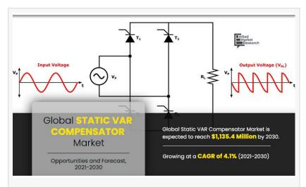
electrical grids. SVCs are a type of power electronics device used to regulate voltage levels and control reactive power in high-voltage transmission systems. With the increasing integration of renewable energy sources like wind and solar, as well as the growing demand for energy-efficient technologies, the demand for SVCs is expected to continue rising.
