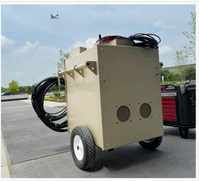
SEMPRE provides a transportable 5G cellular network, an enterprise-level datacenter and a satellite gateway in one EMP-hardened enclosure. Shown at Barksdale AFB, LA.
