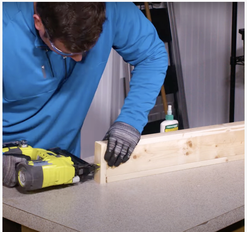
Due to the large quantity of nails, a nail gun is recommended, however a hammer can be used in lieu of a nail gun.
