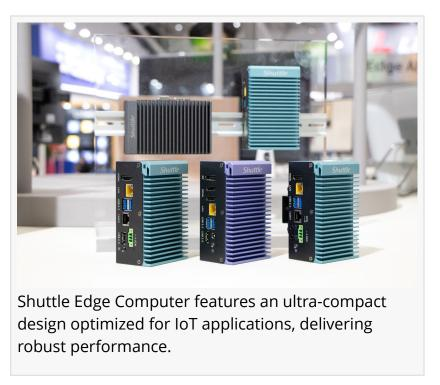
extensive I/O interfaces and high-speed network connectivity. The SPCEL12 model features 2 HDMI ports, 1 DisplayPort, dual Intel 2.5G Ethernet ports, M.2 expansion slots, and USB 3.2Gen2, making it ideal for professional audiovisual integration and edge computing applications.
