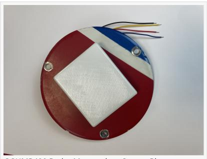
GGHMR400 Radar Mounted on Cessna Plate
