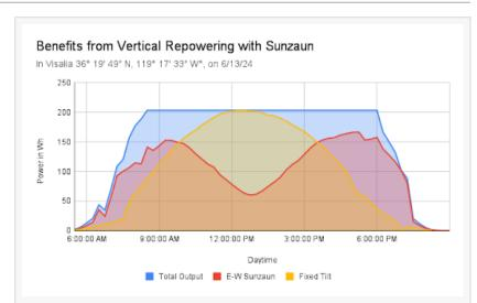
Vertical solar systems can supplement the generation profile of existing south-facing systems. (The irregularities in the red production curve of the vertical east-west system in the morning hours are due to shading of the test array.)
