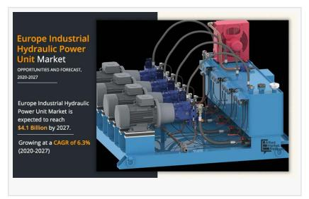
The hydraulic power unit implements the pressure that runs cylinders, motors, and other parts of a hydraulic system. These power units, unlike standard pumps, use pervasive pressurization networks for moving fluid; and comprise temperature control devices. The mechanical specifications and characteristics of a hydraulic power unit defines the kind of projects it will be effective for.
