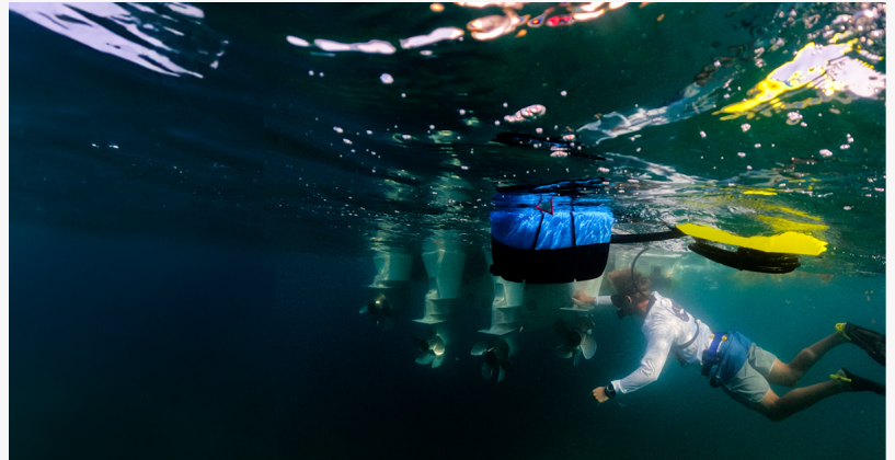
A diver is seen underwater, using the BLU3 Nomad Mini dive system to inspect the propellers of a boat. The Nomad Mini unit floats above on the water's surface, providing air through a hose.
