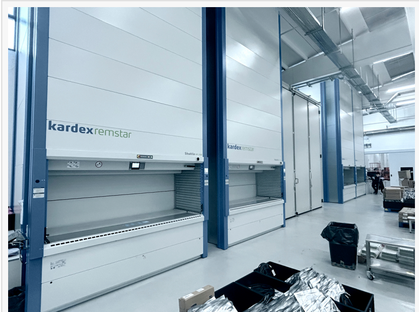
Kardex Remstar designed a solution using 13 Vertical Lift Module Kardex Shuttles, all managed by custom software
