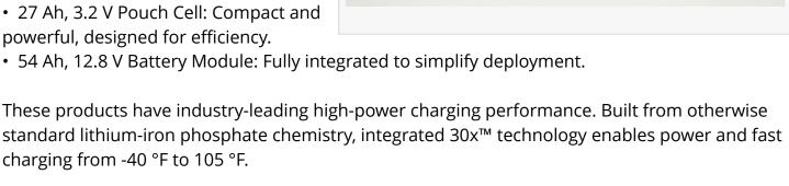
The 12.8 V module stands out with a standard charge rate of 3C (162 amps, 20 min.), achieving thousands of cycles. Additional charger time savings are possible with a maximum continuous
