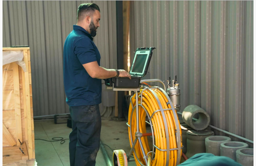
Clean Out Plumbing's Marco Jover using the Dancuter Super Flex robotic pipe cutter
