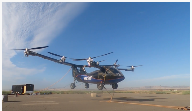
Tethered unmanned flight test ASKA A5 full-scale prototype
