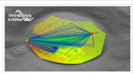
Wireless InSite simulation of coverage and multipath in a lunar crater.
