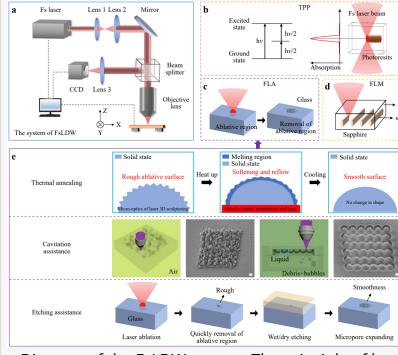
a Diagram of the FsLDW system. The principle of b two-photon polymerization (TPP), c femtosecond laser ablation (FLA) and d femtosecond laser modification (FLM). e Assisted methods for FLA.
