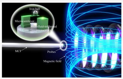
Schematic diagram of the MCF-tip probes for magnetic field and temperature discriminative sensing.
