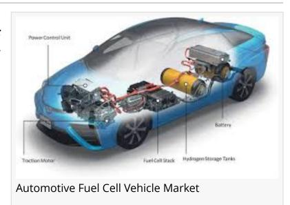
from the air to produce electricity that powers the vehicle, emitting only water vapor as a byproduct. This zero-emission feature makes FCVs an attractive alternative to traditional internal combustion engine vehicles, especially as concerns over air quality and carbon emissions intensify. The market's expansion is being driven by advancements in fuel cell technology, the
