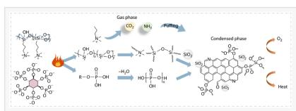
Proposed intumescent flame-retardant mechanism of the P2N2 coating.
