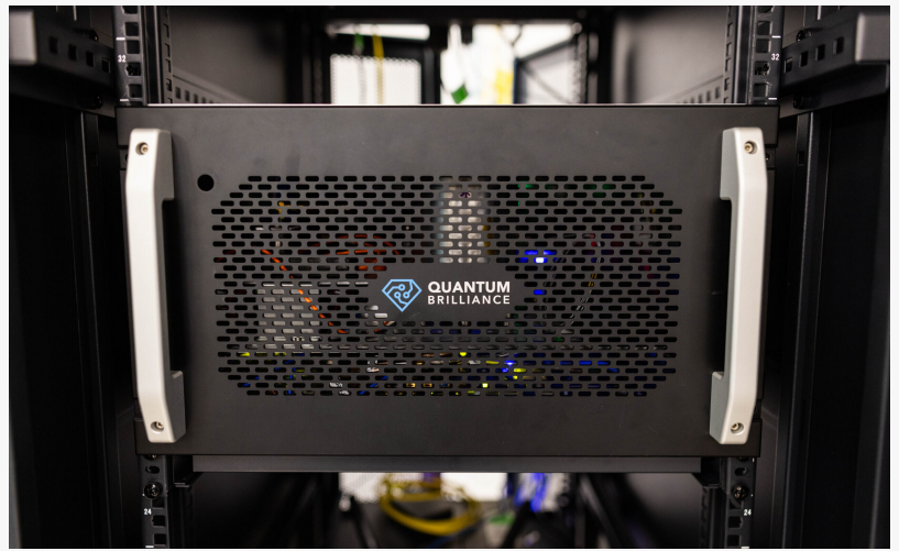
A diamond-based, rack-mountable quantum accelerator from Quantum Brilliance
