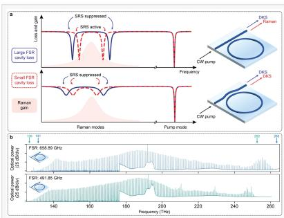
Thin-film lithium niobate microresonator Raman lasing suppression methods and octave-spanning frequency combs
