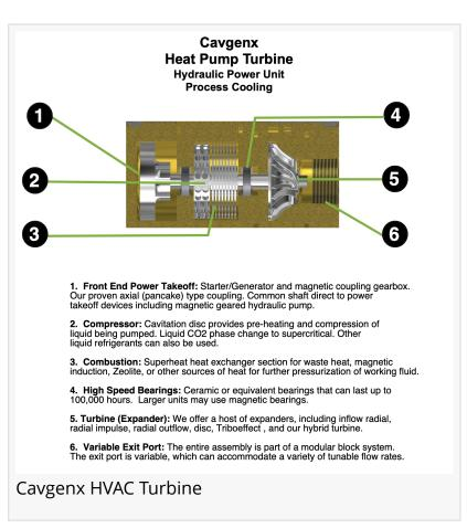
produced by AI GPUs in data centers. This not only reduces the need for external power sources but also significantly lowers the cooling costs traditionally associated with running a data center.
