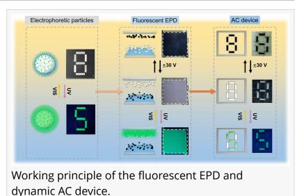
(EPD) has a fast response, dynamically switch image and bright luminescence, providing potential in multifunctional AC applications.
